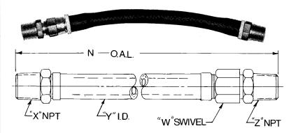
The Standard Cary flex hose assembly includes brass fittings and hose with synthetic rubber liner and cover and one textile braid reinforcement—used for water, air, and oil to 190° F. and 200PSI.
